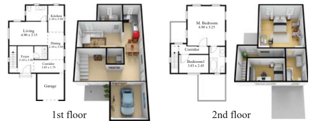
Figure 11: An interior layout of a two-storey house. The stairs are considered as special rooms that should be consistent between two floors. The floorplan of each floor is shown on the left, 3D renderings are shown on the right.
