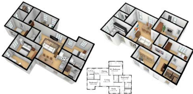
Figure 10: An interior layout of a bungalow-style house generated by our algorithm. The floorplan is shown in the middle. Two sides of the 3D rendering are shown.
